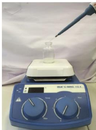
Figure 4. Process of drop by drop to perform emulsion
