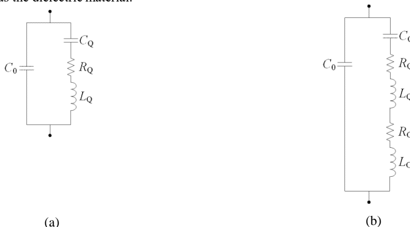
Figure 1. Electrical equivalent model of the QCM sensor without coating (a) and with coating (b)
